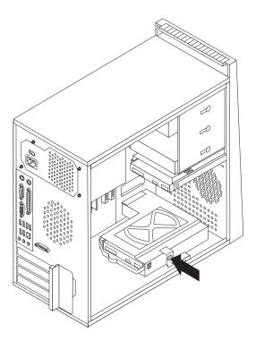
Figure 21. Removing the secondary hard disk drive
